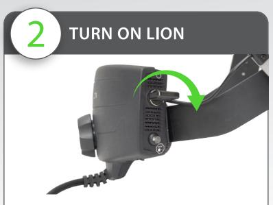
Locate the key switch on right side of the LION. Insert key into key switch and turn on. The light on the back of the LION headset will blink blue as it is establishing connection to the tablet.
