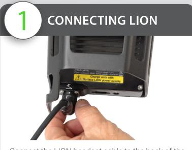
Connect the LION headset cable to the back of the footswitch mating cable receptacle. Please note: this connector is keyed, so it must be inserted in the proper orientation with the arrow on the connector facing up.
